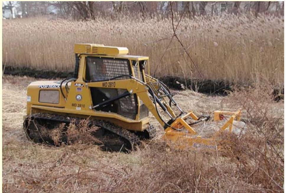
The Posi-Track ASV is a low-ground pressure vehicle used for mowing dead phragmites stems and brush.
