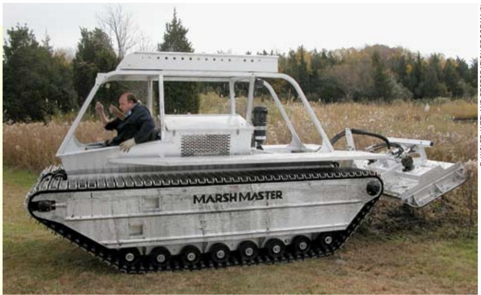
The Marsh Master is an amphibious tracked unit that can be outfitted with a tank sprayer for herbicide applications or used for mowing dead phragmites stems.
