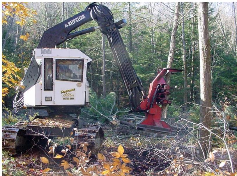
*Figure 6. Feller-Buncher used in the treatment.*
