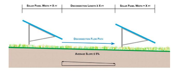
$\frac{Figure \ 2}{Solar Panel Installation with Slopes > 5\% and \le 10\%}$
