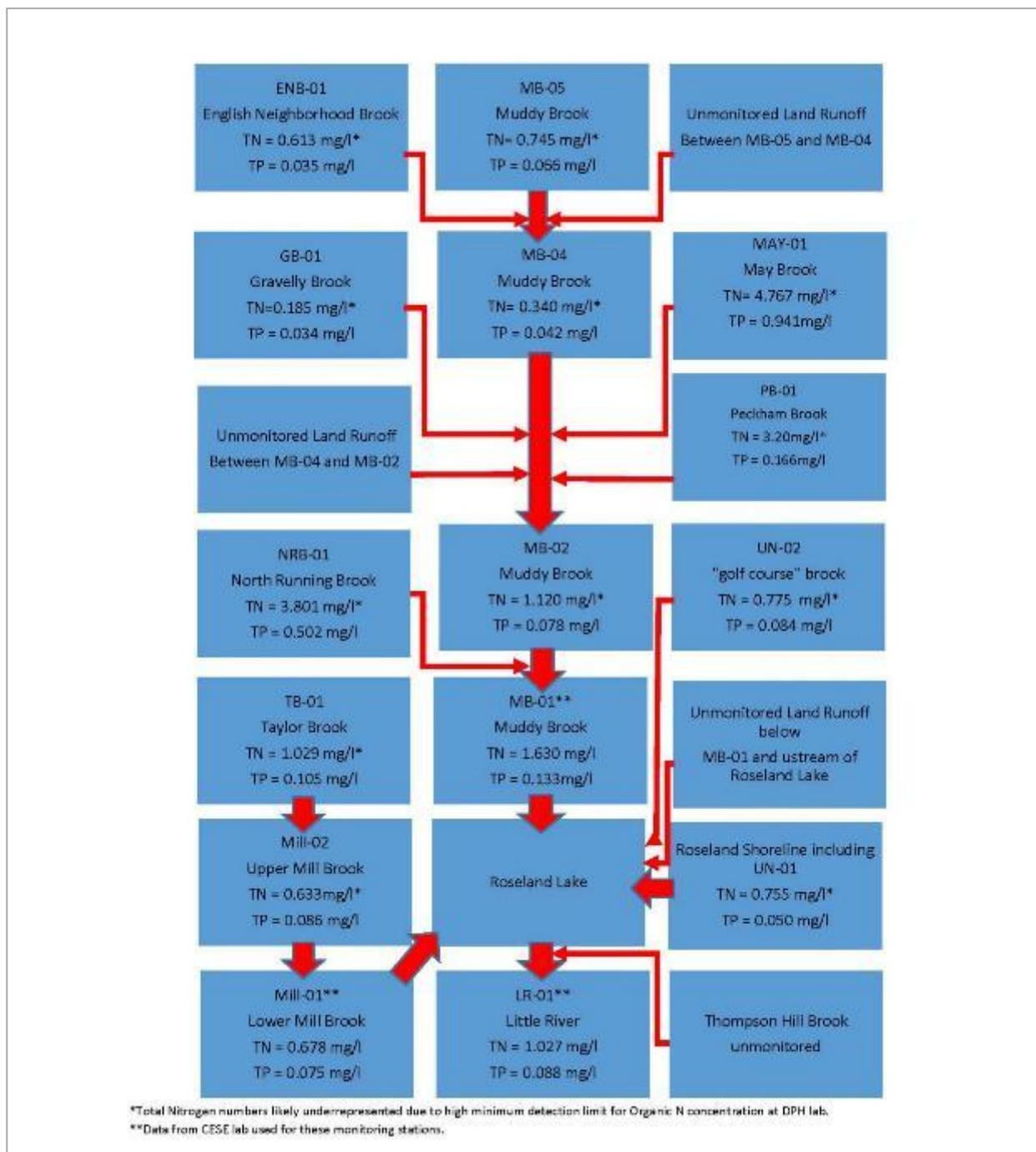
Figure 7: Roseland Lake Nutrient Flow Schematic
