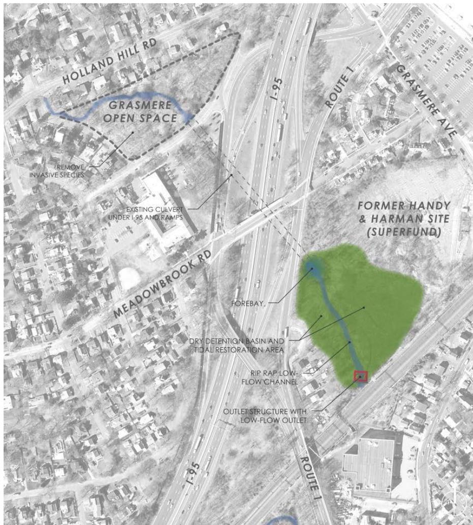
**Figure 4-10. Flood Storage and Tidal Wetland Restoration at the Former Handy & Harman Site**
