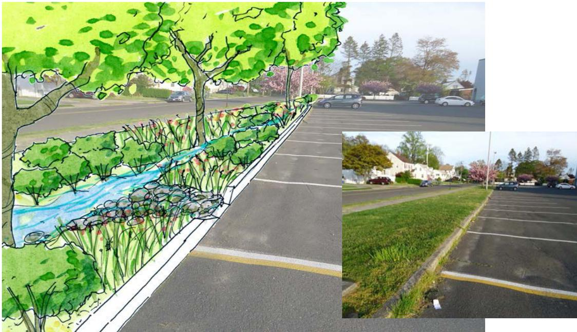
**Figure 4-8. Before and After Concept Design for a Bioretention Area for the Parking Lot**
