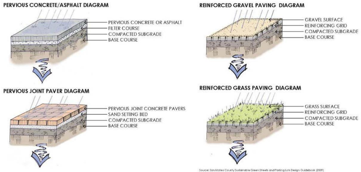
**Figure 4-9. Diagrams of Selected Permeable Pavement Systems**
