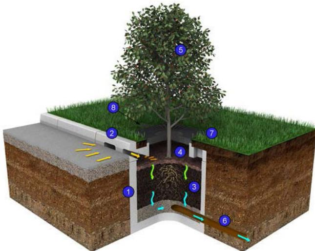
**Figure 4-15. Typical Tree Box Filter (Source: Hydro International, Inc.)**
