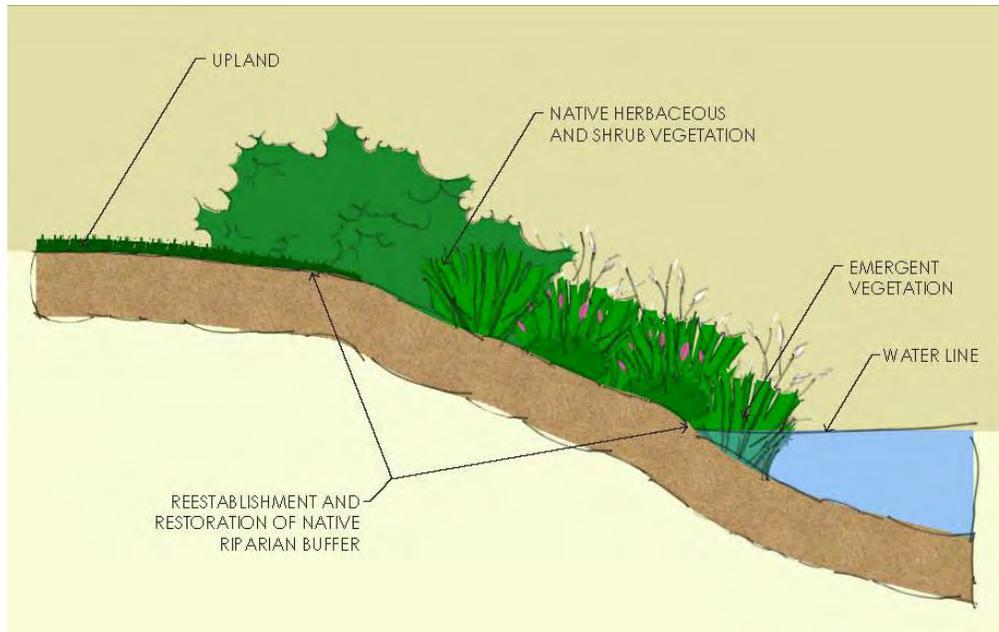
**Figure 4-5. Typical Bank Restoration Planting for Small Streams**
