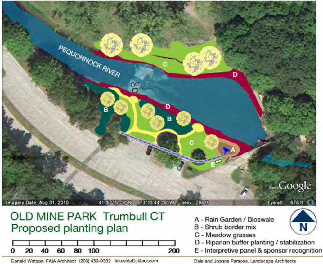
Figure 4-22. Old Mine Park Restoration Concept Site Plan
