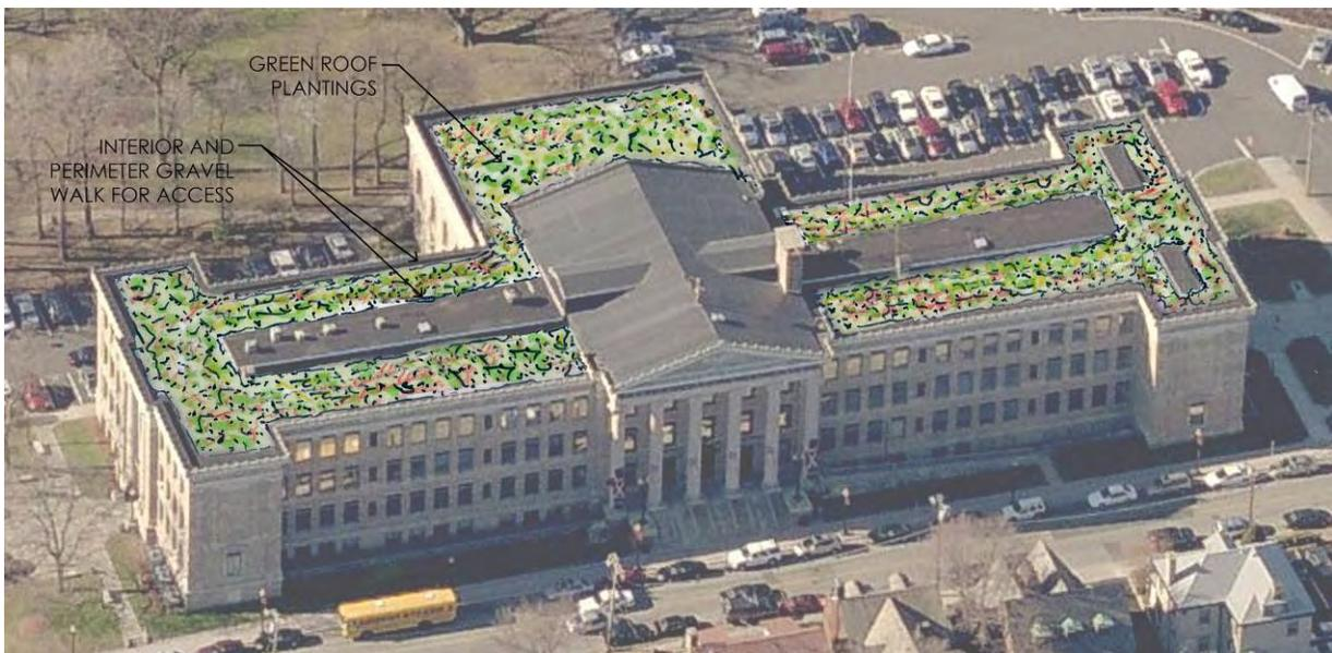
**Figure 4-14. Bridgeport City Hall Green Roof Retrofit Concept**
