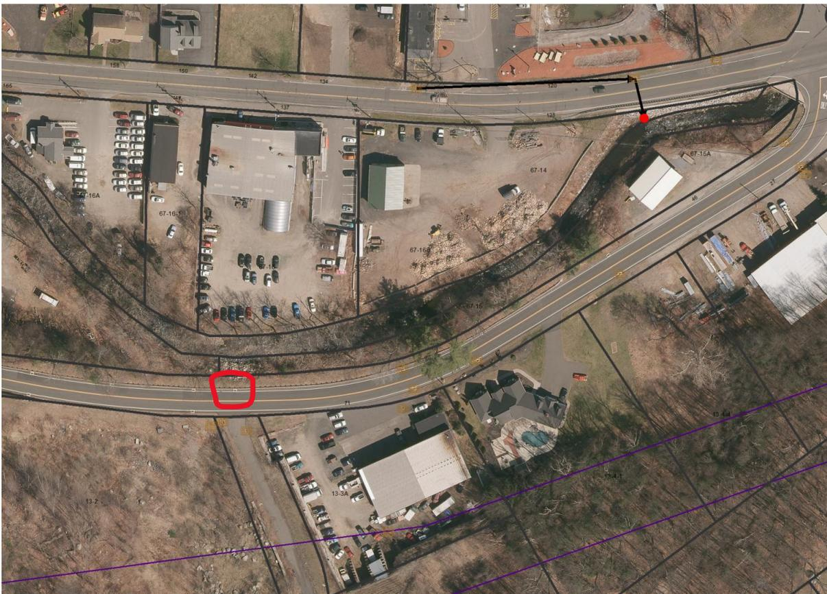
The open circle indicates the location of a Vortech unit, which removes and stores sediment, prior to the storm water draining into the Pequabuck River. Sedimentation basins, such as the Vortech unit require periodic cleaning to remain effective.
