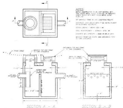
**SEDIMENTATION STRUCTURE DETAIL**
