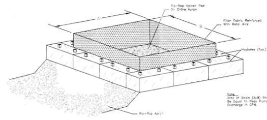
Temporary Sediment Basin For Dewatering Discharge N.T.S.
