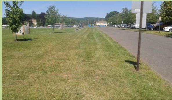
**Pervious Pavement.** 15,000 square feet of pervious pavement is proposed for the middle two rows of parking in the north parking lot. This conversion to pervious pavement would reduce the impervious surface of the 50,000 square feet lot by nearly 30% and decrease the volume of stormwater inputs to the existing drainage system. *Estimated Cost: \$60,000*
