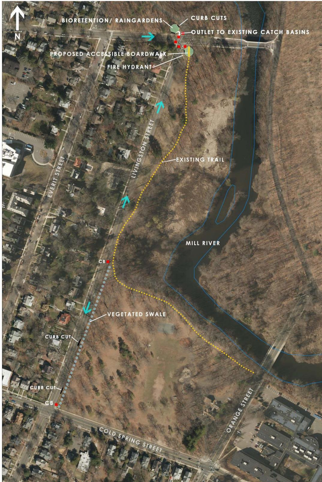
Figure 18. Proposed green infrastructure retrofits for Livingston Street at East Rock Road. "CB" indicates existing catch basin. Blue arrows indicate existing surface flow patterns.
