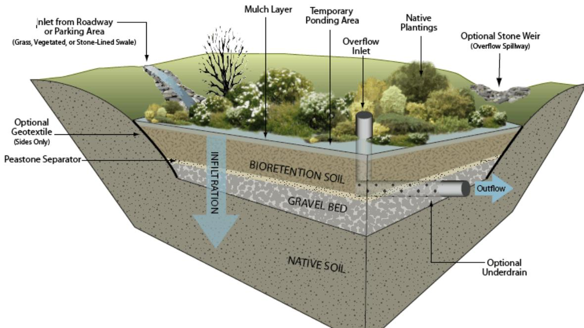
Figure 10. Bioretention schematic.
