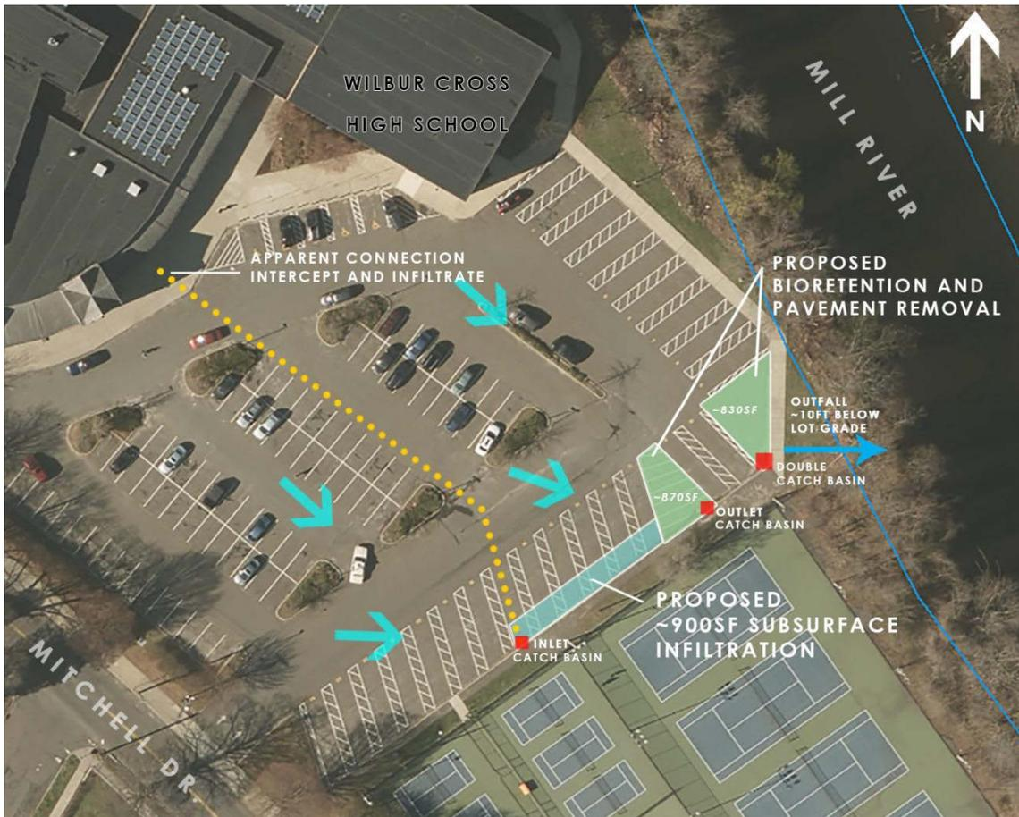
Figure 13. Proposed green infrastructure retrofits for Wilbur Cross High School. Red squares indicate existing catch basins. Blue arrows indicate existing surface flow patterns.
