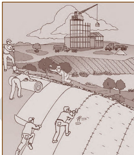
Figure 5- 13 Example of Temporary Erosion Control Blanket Installation
