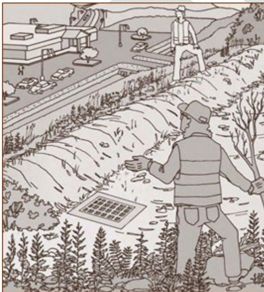
Figure 5- 52. Illustration of Permanent Diversion Intercepting Overland Flow
