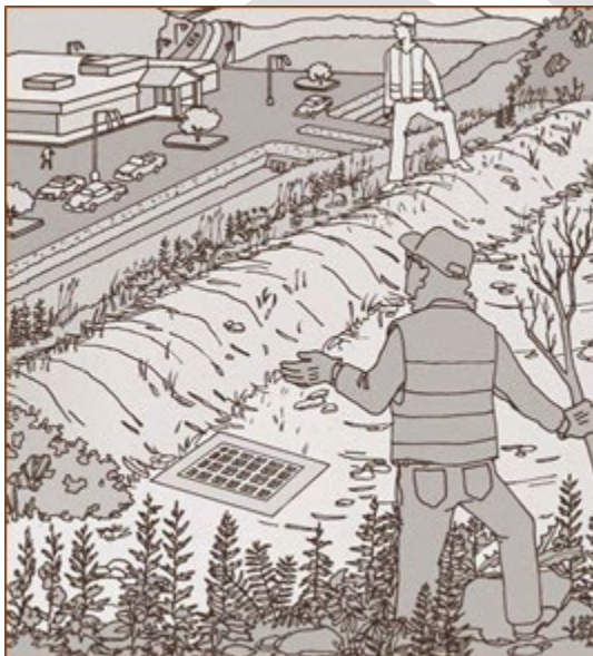
Figure 5- 52. Illustration of Permanent Diversion Intercepting Overland Flow
