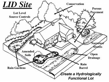
Figure 3.1 – Schematic of engineered practices.
