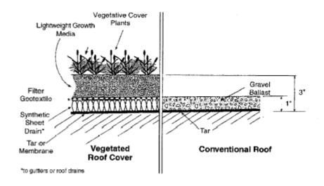
Figure 4.23 - Example Vegetated Rooftop Cross-Section
