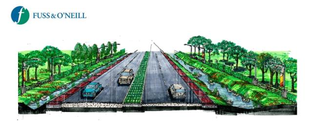
Figure 3.9 - Shoulder Treatment Systems using detention and filtration design.
