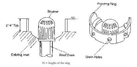
Figure 4.22 – Roof ponding rings. Source: Tourbier, 1974.
