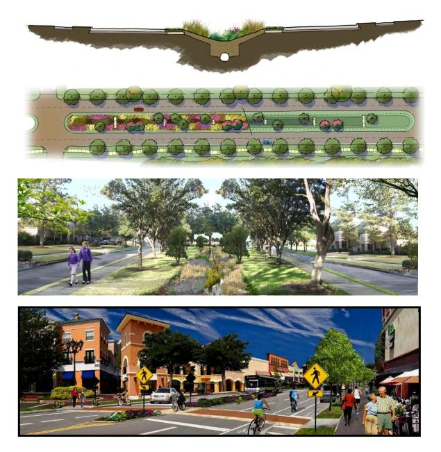
Figure 3.8 – Examples of center median infiltration/filtration systems
