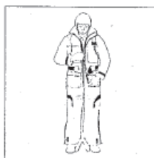
2. Close chest and leg zippers with a slow even pull. Secure velcro storm flap.
