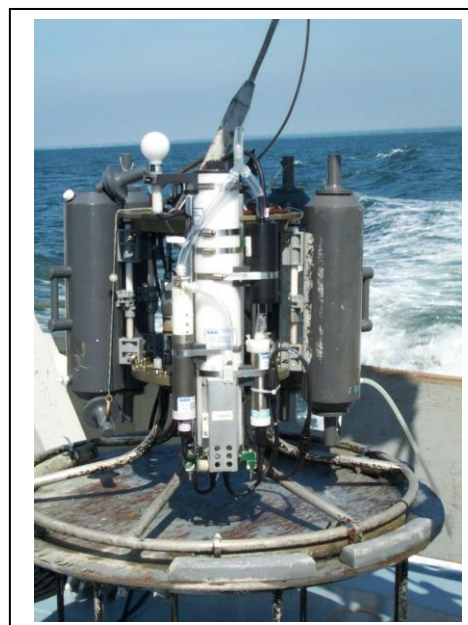
Figure 4. Rosette, CTD, and Niskin sampling array
