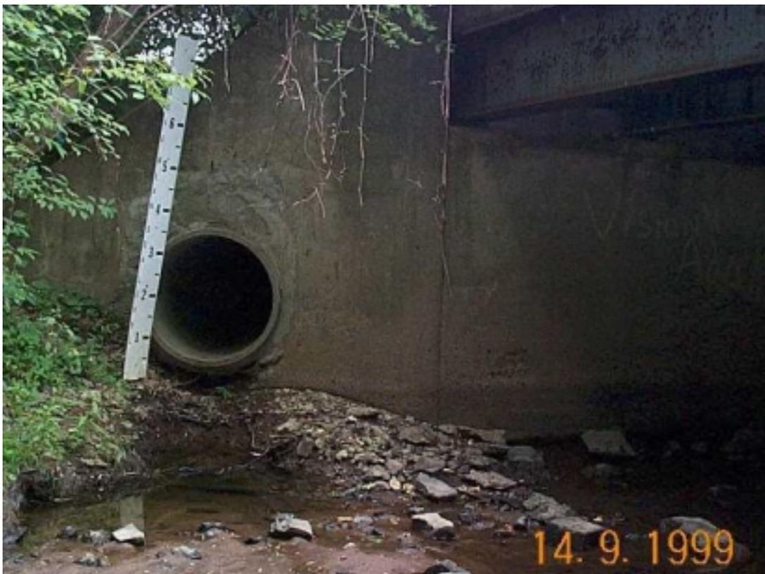
*Farm River, East Haven, CT, August, 1999. Poorly constructed gaging station at a registered diversion. The staff gage is high and dry even though there is water in the channel, and the staff is leaning over, making any data collected from this gage inaccurate.*
