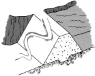
Creates areas bare of erosion protection and causes erosion channels. Allows water to stand and makes area susceptible to drying cracks.
