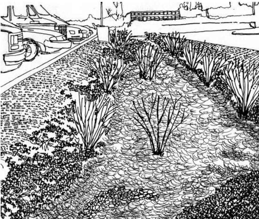
Figure 2.1. Curbless perimeter bioretention
