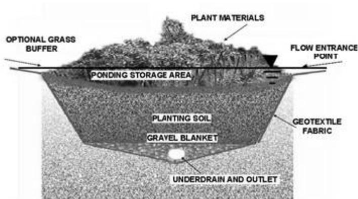
Figure A.3. Bioretention components
