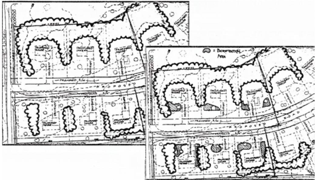
**Figure 4.4. Example site plans with and without bioretentions**
