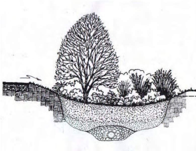
Figure 2.14. Filtration/partial recharge facility
