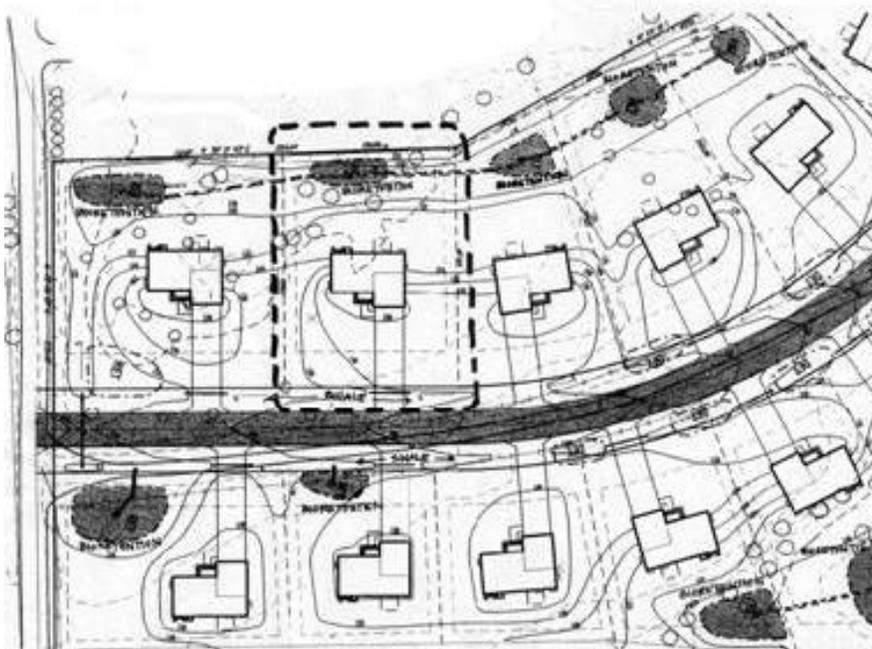
Figure 3.2. Typical site plan with bioretention
