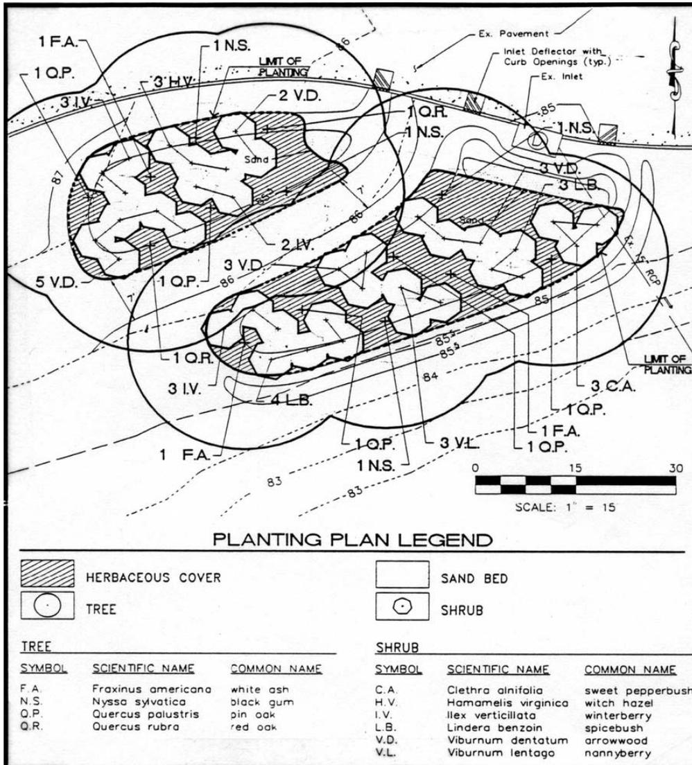
Figure 5.1. A typical bioretention landscape plan
