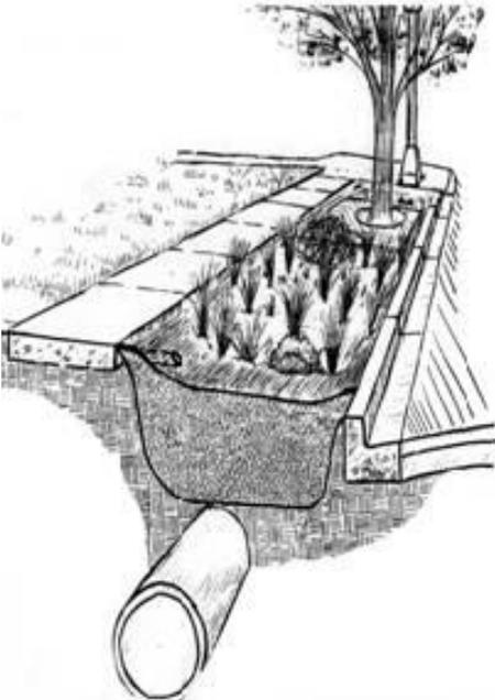
Figure 2.11. Tree-box area bioretention
