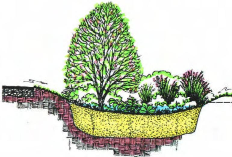
Figure 2.13. Infiltration/recharge facility (enhanced infiltration)
