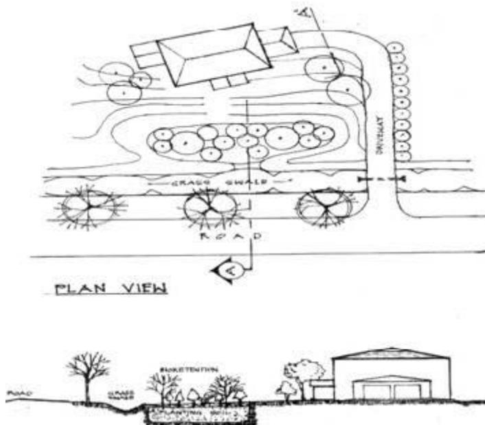
Figure 2.6. Plan view and cross section of a swaleside bioretention area
