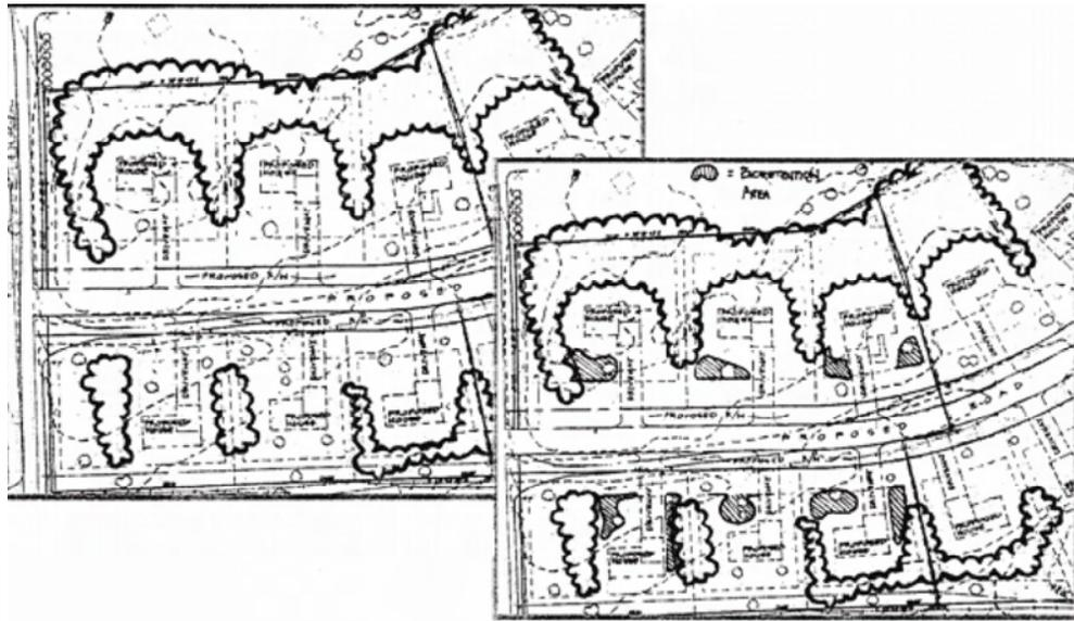
Figure 4.2. Proposed site plans without and with bioretention
