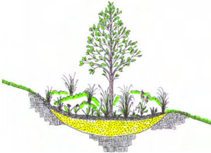
Figure 2.9. Shallow dish (scalloped) bioretention
