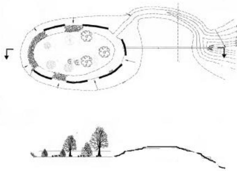
Figure 2.2. Curbless *flow-through* bioretention
