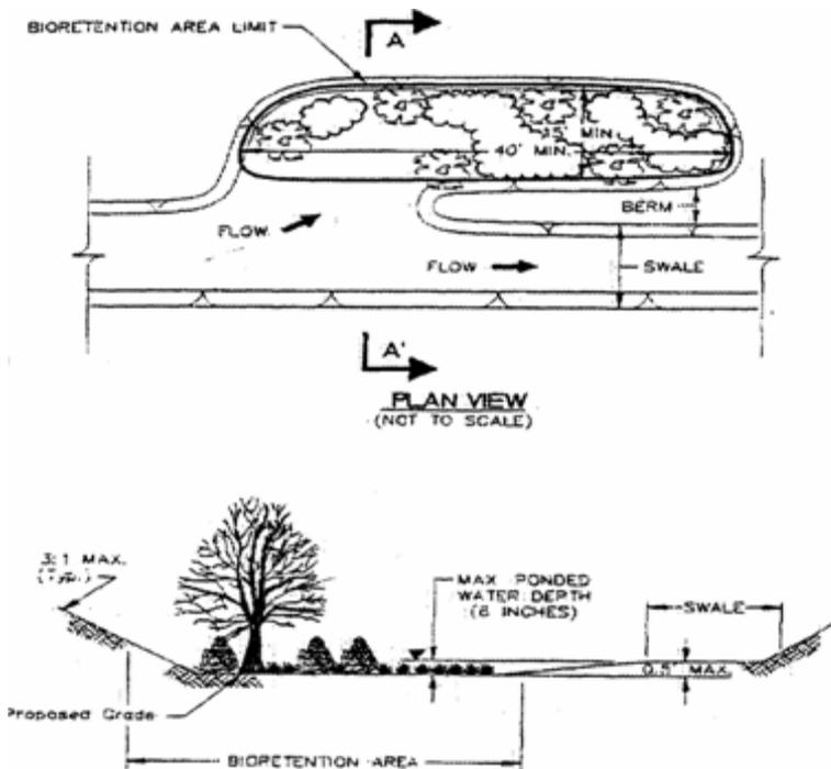
Figure 3.1. Offline bioretention
