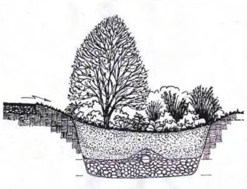
Figure 2.15. Infiltration/filtration/recharge
