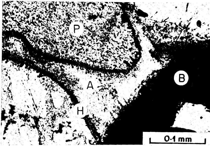
Fig. 18. Buckland brownstone with albite (A) cement that fills former interstitial pore. Mechanically trapped silt and clay float in the albite cement. Hematite (H) rims the detrital grains, including altered detrital plagioclase (P). The biotite flake (B) is almost completely altered to hematite.
