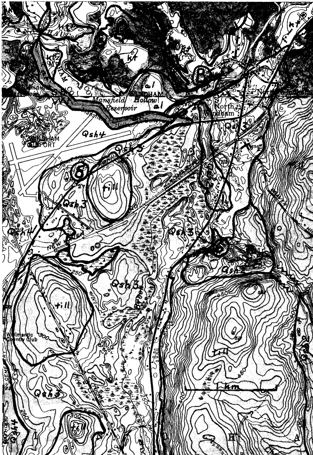
Figure 4.- Part of Spring Hill (SH) and Willimantic (WI) Quadrangles, showing Stops 5 and 6 and Optional Stop B. Glacial deposits generalized after Rahn (1971) and Clebrik (1980) respectively. Qsh2-4 are morphosequences, ic is ice contact, kt is kame terrace, k is kame, al is alluvium, and af is artificial fill.
