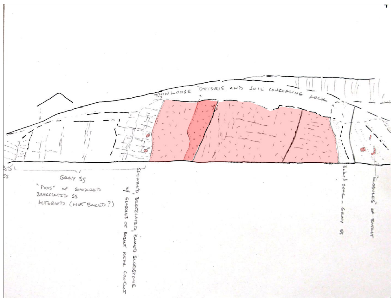
Figure VII-6A. Patten Road cut (area 104 looking southeast). Photograph, approximately 10 m in height, of dikes of West Rock diabase. Schematic drawing of same, with diabase shaded light pink for older dike and darker pink for columnar jointed younger dike (yellow box shows approximate area of text figure 12A). Gray sandstone to east (left) of dike is faulted. We infer that hydrothermal fluids flowing through the fractures altered the sandstone to produce dark gray color. Relict bedding is dips toward west at low angles. Reddish-brown sandstone on east (far left, that) dips 22 degrees west; this is interpreted as drag caused by down-to-the-west faulting. Reddish-brown sandstones on west side dip more steeply to west; this is interpreted as normal drag along the fault system.
