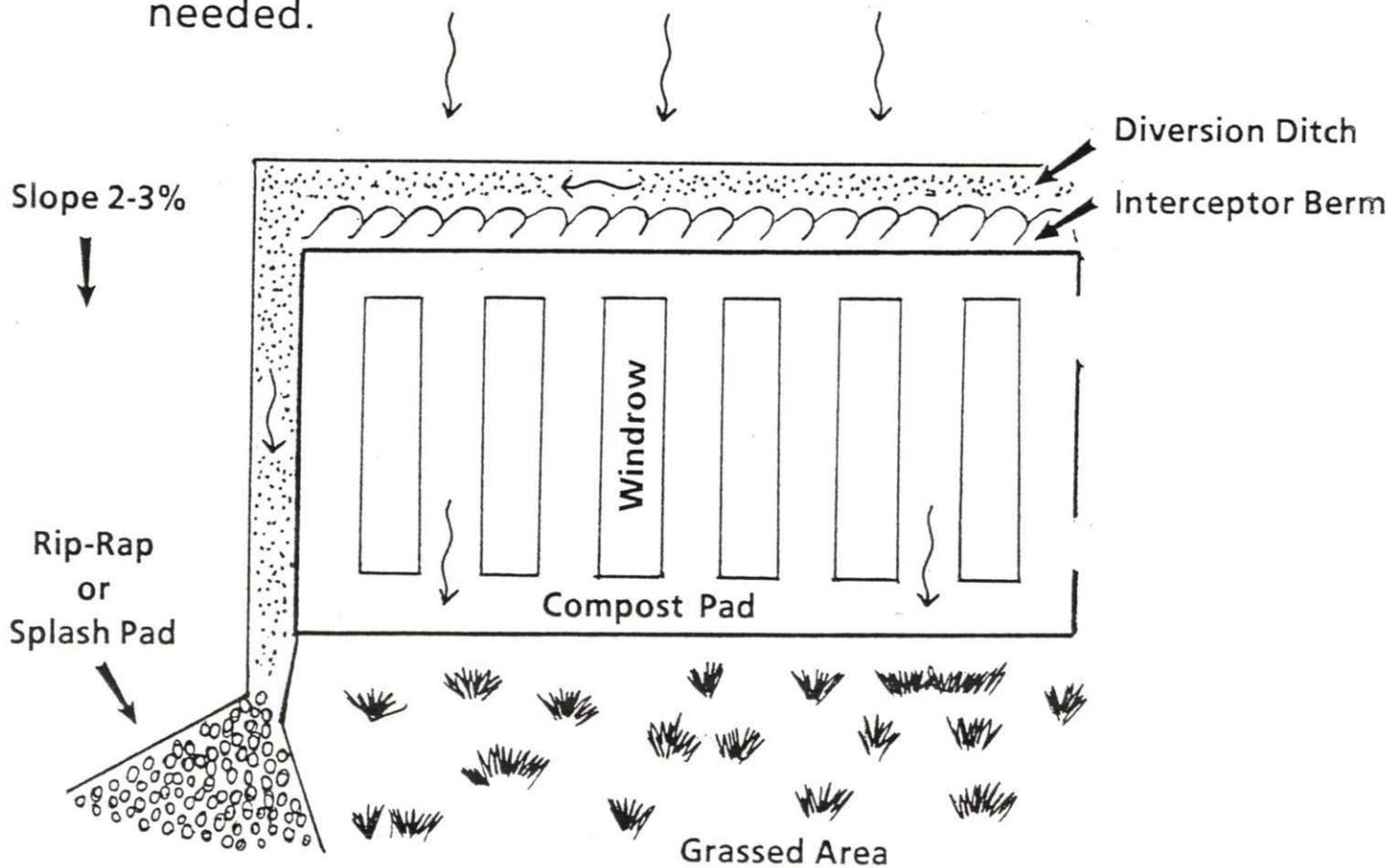
Generic Site Plan to Control Run-off and Run-on
