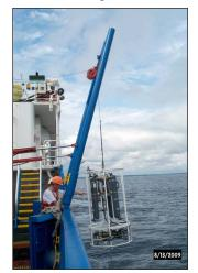
CTD (conductivity/temperature/depth) monitoring array is deployed from OSV Bold
