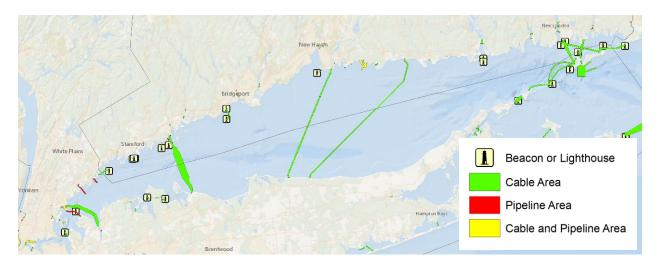
Figure 26-3: Major Cable infrastructure and Lighthouses in Long Island Sound. Pipeline areas were included in this map graphic, due to the Y50 cable being designed as a Pipeline Area in the NOAA ENC. This map is a combination of spatial information from a variety of different sources, including NOAA Electronic Navigation Charts and the Northeast Ocean Data Portal (NOAA, 2018; Northeast Regional Planning Body, 2018).
