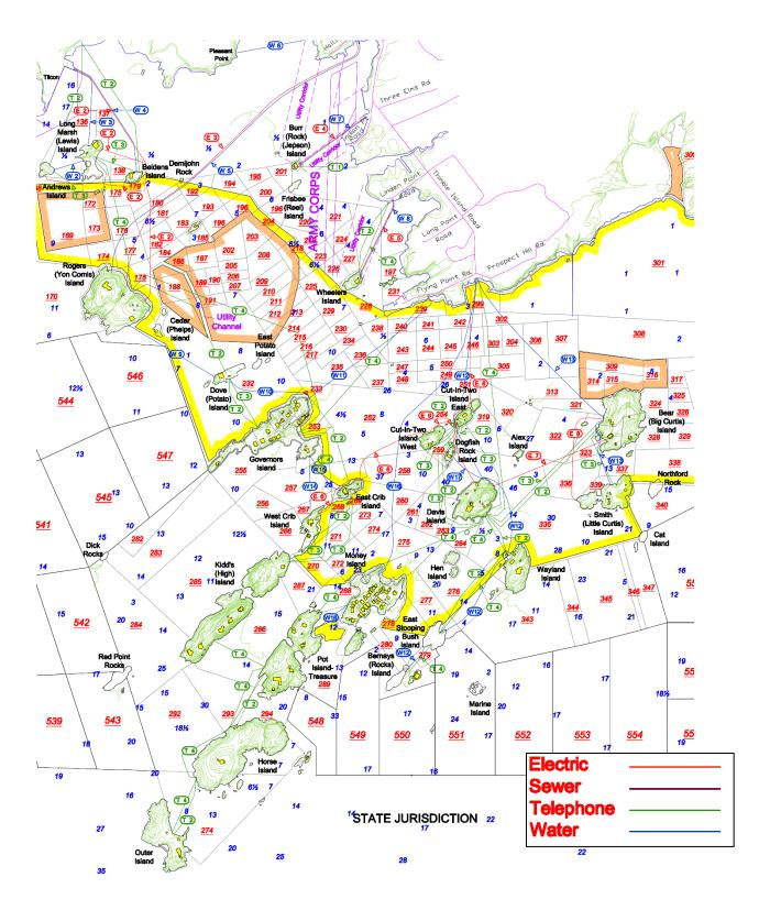
Figure 26-2: Cables and Pipelines Surrounding the Thimble Islands. The Town of Branford has mapped out, among other things, the electric and telephone cables and the water and sewer pipelines running between and to/from the Thimble Islands. Electric cables are owned by the
