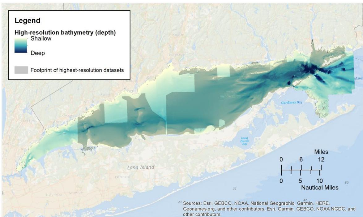
Figure 4. 8-meter horizontal resolution bathymetry mosaic for Long Island Sound. The highest resolution datasets within the Blue Plan planning area are shaded in grey.
