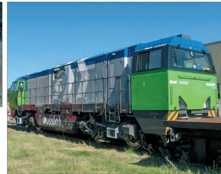
G2000, mainline locomotive with 2700 kW with particle filter and regeneration system
