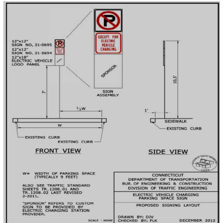
The pavement of the EV parking spot should be painted to clearly indicate to others that the spot is designated for electric vehicles. Pavement markings, similar to striped markings used for spaces reserved for handicapped parking; as well as markings on vertical surfaces should be used to identify EV charging spaces. Often times both a parking spot and a curb is painted to identify a spot designated for EVs.
