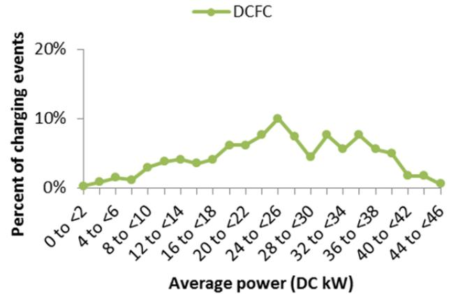
**Figure A2. Distribution of average power per charging event for the DC fast charger.**
