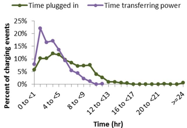
Figure A10. Distributions of time connected and time transferring power per charging event for Level 2 charging events with average power of 5.6 kW or greater.
