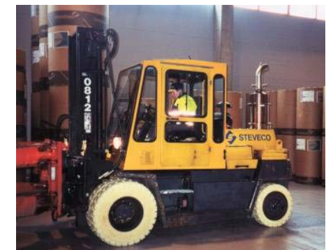
Lift truck retrofitted with DPF
