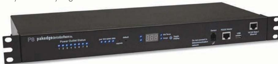
The Pakedge P8 and P8E are equipped with an Auto Ping Server. It pings each device every 1.5 seconds and if the PDU does not receive a reply back it will power cycle the device. It then sends an email to both the end user and dealer informing them of the event and that the issue is resolved. This innovative feature will save you time and money!
