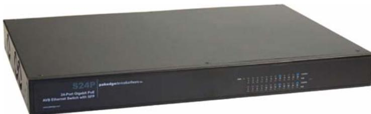
With its massive 390 Watts power supply, the S24P can provide Ethernet and power to devices that are 802.af-compliant. Each of the 24 ports can deliver up to a full 15.4 Watts of power. In addition, each port can be power-cycled individually if a connected PoE device becomes unresponsive or needs to be rebooted.
