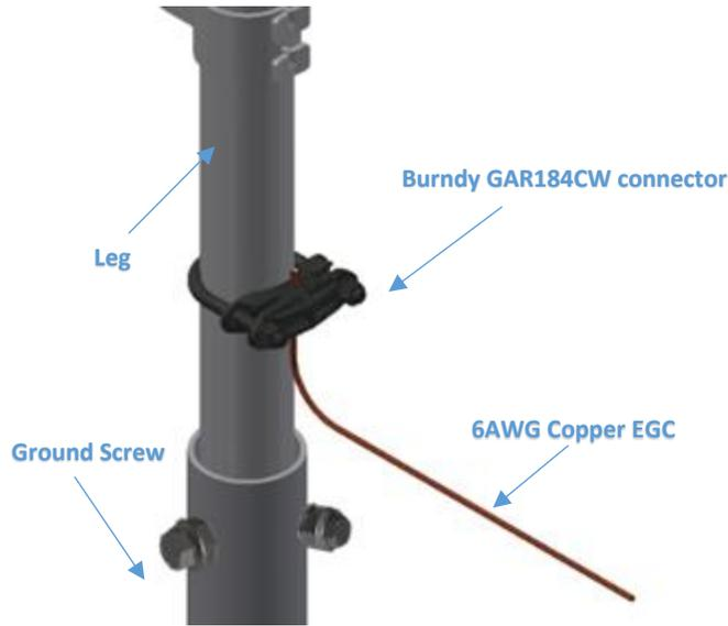
**Figure 3.4.3 View of Grounding Clamp on Table Post**
