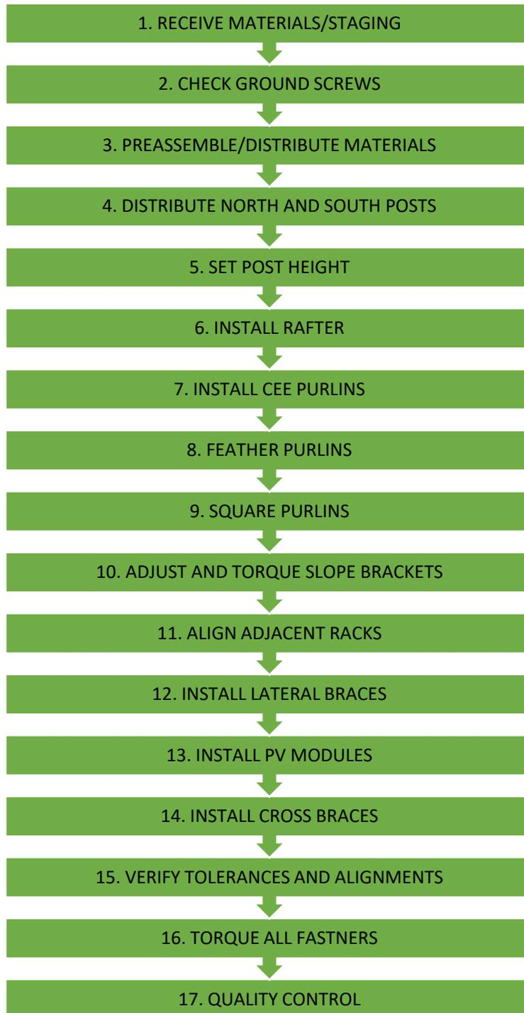
**Figure 3.2.1 Suggested workflow for the TerraGlide Landscape Mounting System installation.**
