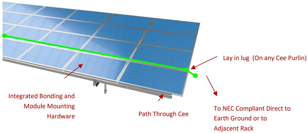
**Figure 3.4.2 Front View of Grounding Diagram**
