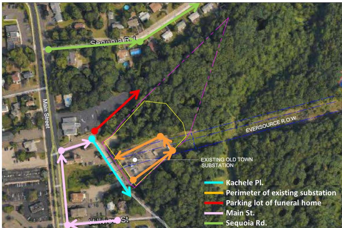
Figure A1. EMF Measurement paths around Old Town Substation.
