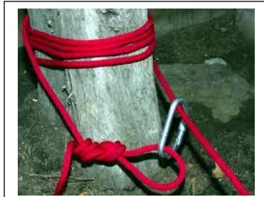
An anchor is the means of securing the ropes and/or system to something solid. Anchors can be natural elements such as trees or rocks, artificial, such as beam clamps or removable swivel bolts or they can be man-made such as structural beams and apparatus.
