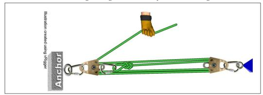
Simple 5:1 Mechanical Advantage using Double Pulleys with a Change of Direction
