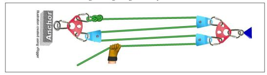
Simple 4:1 Mechanical Advantage using Double Pulleys with a Change of Direction
