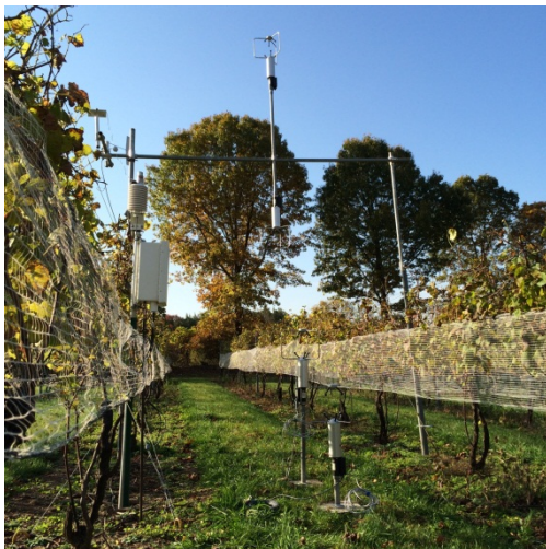
←3D-sonic anemometers measure wind information in a Pinot Gris vineyard at Lockwood Farm in Hamden, CT.
