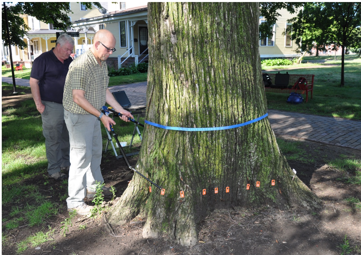
Dr. Marra measuring the geometry at the base of an American elm, in preparation for tomography. Governors Island, New York.
