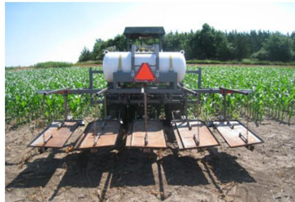
**A tractor mounted flame weeding unit, developed at the University of Nebraska-Lincoln**
