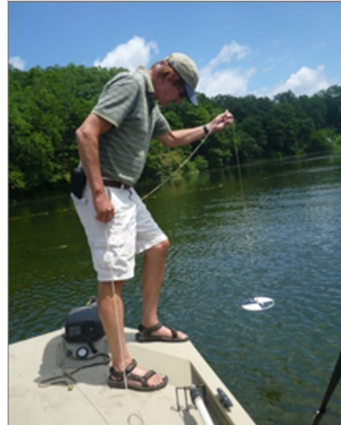
Figure 3. Checking water clarity with Secchi disk.
