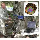
are using new technologies that employ sound waves and electrical currents to quantify internal decay in living trees and its role in carbon
