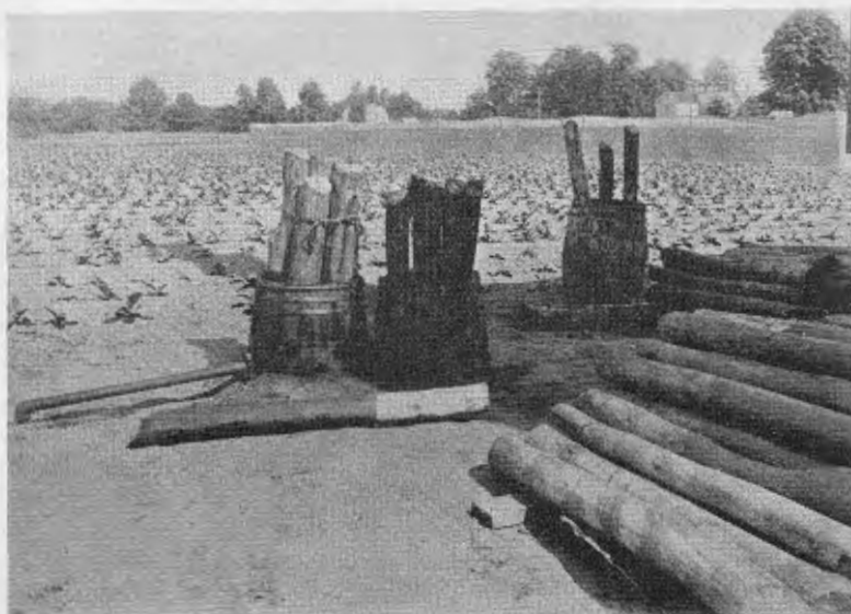
FIGURE 68. Simple equipment for treating poles by the open tank method. Creosote in barrel on left is heated to 220° F. by charcoal fire in pit under end of 2 inch pipe return coil. Cold creosote bath in second barrel. Third barrel is for draining excess creosote. Tops of poles cut off in this experiment.
