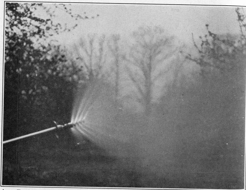
b. Delivery of spray from the nozzle shown in a. Note the solid cone-shaped whirling spray which covers the tree with great rapidity. Absence of projections on the end of the spray rod to catch on branches is a decided advantage. It can be thrust into the center of a tree covering parts not ordinarily reached with the usual spray outfit.
