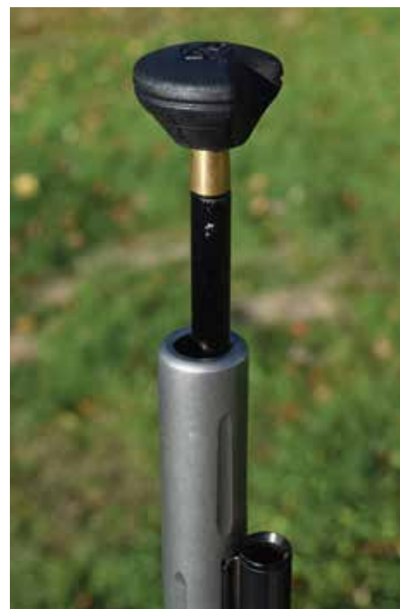
(Right) A muzzleloader must be loaded separately with a powder charge and projectile from the muzzle end of the gun. The ramrod is used to press each component down into the barrel.
