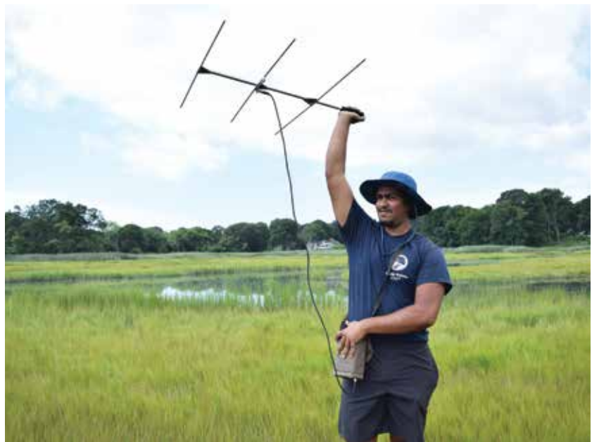
DEEP Wildlife Division field technician Kavi Khadar is using telemetry gear to pick up the radio signal of a nearby terrapin fitted with a transmitter. Weekly trips to this saltmarsh are required to keep tabs on the individuals being studied.
