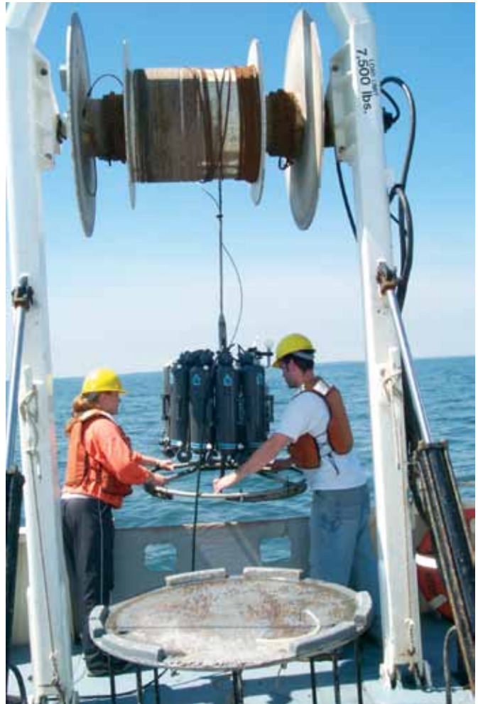
The Water Quality Survey team deploying an instrument array off the CT DEEP research vessel John Dempsey . A summary of the data gathered in the Survey is available on the DEEP website at www.ct.gov/deep/lib/deep/water/lis_water_quality/hypoxia/2013_season_review.pdf .
