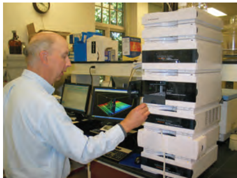
DR. WALTER KROL using LC-FLD to analyze seafood samples taken from areas impacted by the 2010 Deepwater Horizon oil spill.
