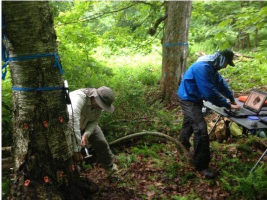
Figure 1. Drs. Marra (left) and Brazeel taking sonic tomographic measurements on a yellow birch at Great Mountain Forest, June 2014.
