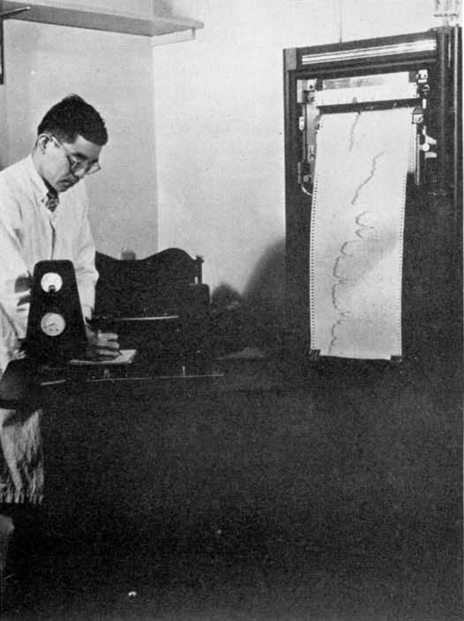
Dr. Tamura notes results of an x-ray spectrometer analysis of a Connecticut soil. Before the use of this instrument, it was impossible to identify the clay particles of a soil, which are largely responsible for its chemical and physical properties.
