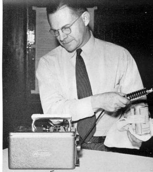
Chemist Richard T. Merwin demonstrates what his duties might be in the event of an atom bomb attack. With the portable Geiger counter, he could determine immediately whether or not a sample of food or water is radioactive.
