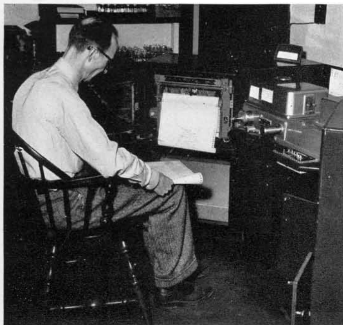
The infrared spectrometer, operated by W. T. Mathis, would be an invaluable tool if war should come to Connecticut. The instrument can identify unknown chemicals, such as might be used in gas warfare, with great speed.
