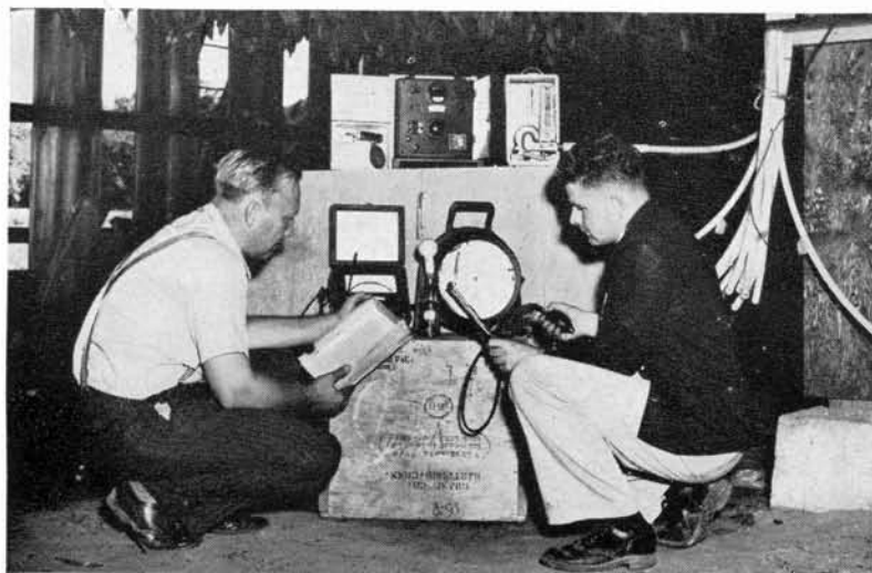
Temperature, humidity and air movement in typical curing sheds are all carefully measured as part of the studies. Left, W. A. Junnila; right, A. B. Pack.
