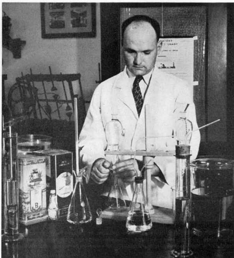
Alphonse Wickrowski is making a separation of squalene, one of the components found in greater amount in olive than in any other edible vegetable oil. A low squalene value indicates little or no olive oil in blends.
