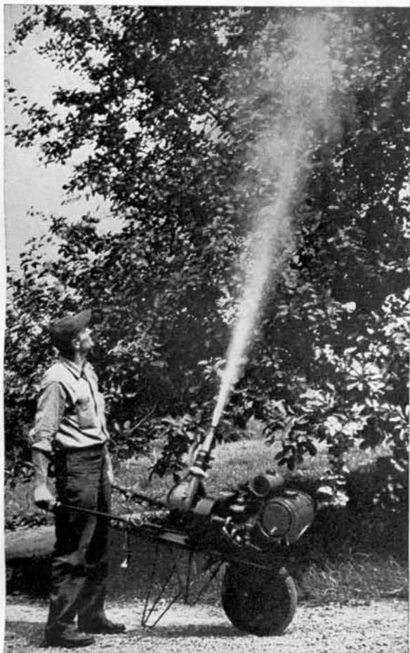
Roderick A. Spencer, one of the designers of the small mist blower shown here, uses the wheelbarrow model for spraying an orchard tree. The model is not adapted for general orchard use but can be used for treating a few small trees.
