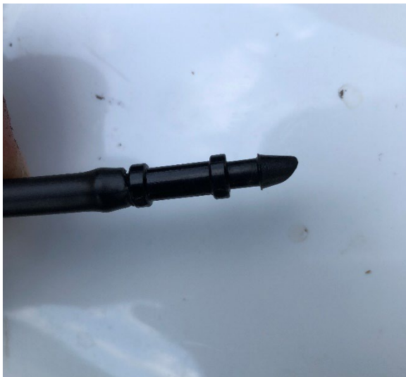
Figure 9. Close up of the ¼” barb connector on the end of the leader.
