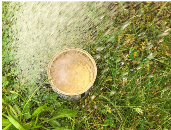
Figure 3. The marked can set under the sprinkler spray.
