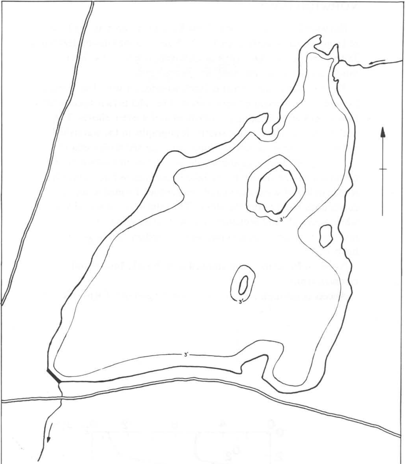
NORTH FARMS RES. WALLINGFORD, CONN. TRACED FROM AERIAL SURVEY MAP 62.46 ACRES PLANIMETER MEASUREMENT CONTOUR INTERVAL 3 FEET 0 1 2 3 SCALE 1" = 300'
