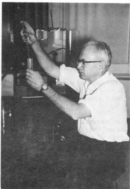
Lloyd G. Keirstead performs a clean-up procedure during a pesticide residue analysis.
