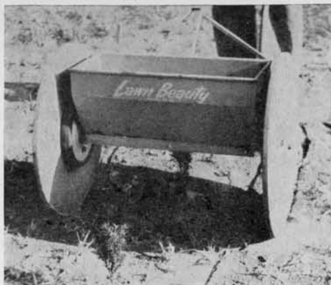
Figure 6. Lawn spreader, with large wheels cut from marine plywood, used to apply granular herbicides in the nursery.
